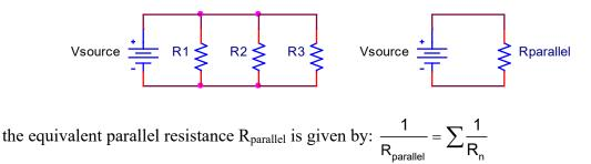
Key properties of a parallel circuit are (1) the voltage across all elements is the same and (2) the currents through all elements must add up to the source current, according to Kirchhoff's Current Law (KCL):
