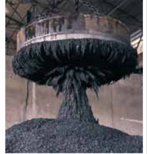
Fig. 28-1 Using an electromagnet to collect and transport scrap metal at a steel mill (Digital Vision/Getty Images)
