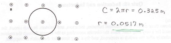
a) What is the magnitude and direction of the induced emf if the magnitude of the magnetic field decreases at a rate of dB/dt = -0.400 T/s?
