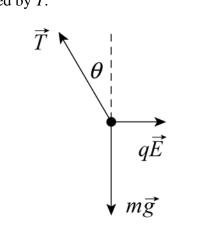
The electric field produced by the plate is normal to the plate and points to the right. Since the ball is positively charged, the electric force on it also points to the right. The tension in the thread makes the angle  $\theta (= 30^\circ)$  with the vertical.
