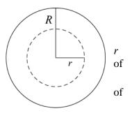
If  $\rho$  is positive, the electric field lines are radially outward, normal to the Gaussian surface and distributed uniformly along it. Thus, the total flux through the Gaussian cylinder is  $\Phi = EA_{cylinder} = E(2\pi r\ell)$ . Now, Gauss' law leads to
