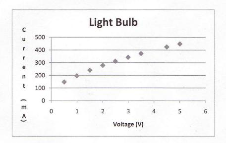
The light bulb did not obey ohm's law and is non-ohmic. The graph of current vs. voltage proofs that the light bulb is non-ohmic because it does not follow a linear path. The light bulbs filament is not constant because of the heat created by the light.
