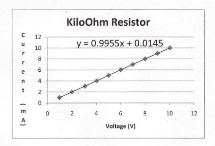
Reversing the polarity of the voltage across the resistor did not make a difference in the current. Graphing the current vs. voltage proved that the  $1k\ \Omega$  resistor is ohmic. Having the graph linear proofs the resistance is constant and therefore, current is proportional to its voltage.
